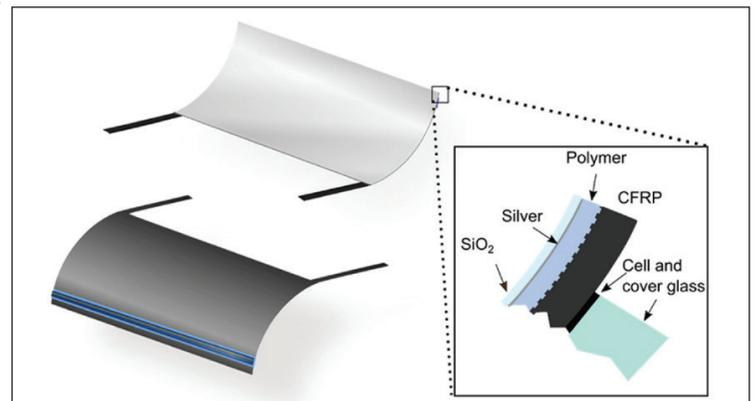
**Figure 1. Schematic of linear concentrator design CFRP backbone is coated in a smoothing polymer (Master Bond UV22DC80-1), silver mirror, and high emissivity SiO<sub>2</sub> layers.<sup>1</sup>**
